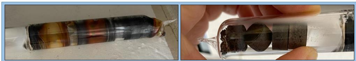
Figure 4. Composite materials sintered in a quartz tube
