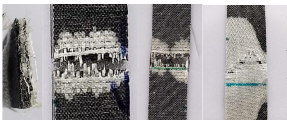
Fig. 4 The damaged digital sample photographs after the tension tests
